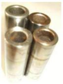
Never mind that inside the pistons we found 3 different gudgeon pins: That would have rather been an unbalanced motor!
