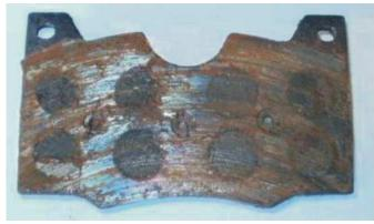
Above: Here we can see that the pad was home-made clearly in an attempt to cut costs, corners, and maybe lives as well, but that is not enough, why do we see the grinding marks at the BACK of the pad, on the metal backing? Bingo...
