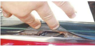
The beauty is that the rubber provides a valve effect, so pressurized air can escape the cabin, but not vice versa.
